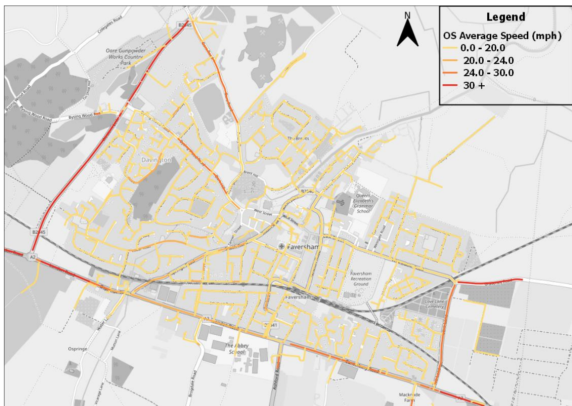
Figure 7: Map showing 20-hour average speeds in Faversham according to OS MasterMap data
