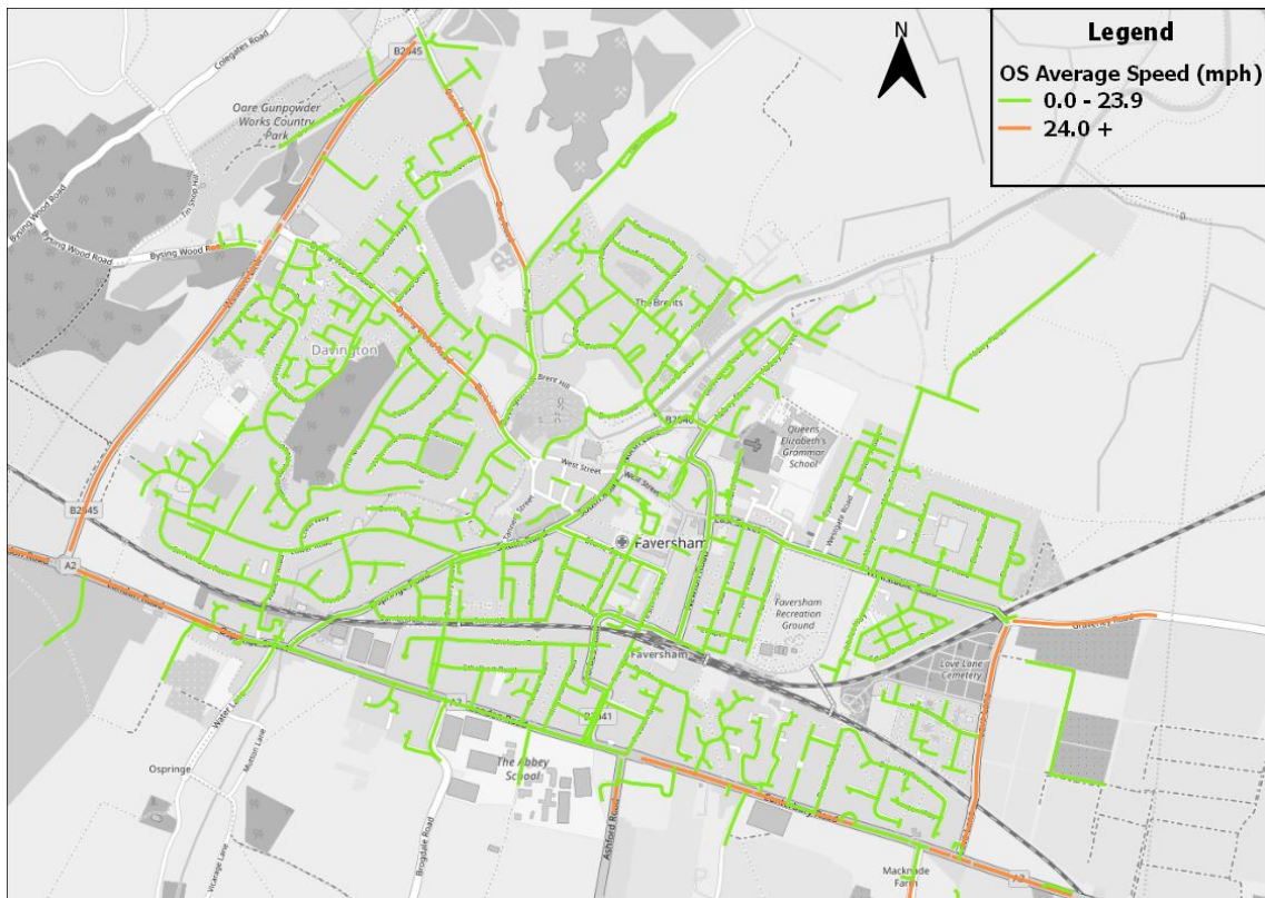
Figure 8: OS MasterMap average speeds categorised above or below 24mph threshold
